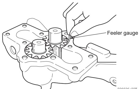
Measuring the oil pump gear-to-pump cover clearance.
