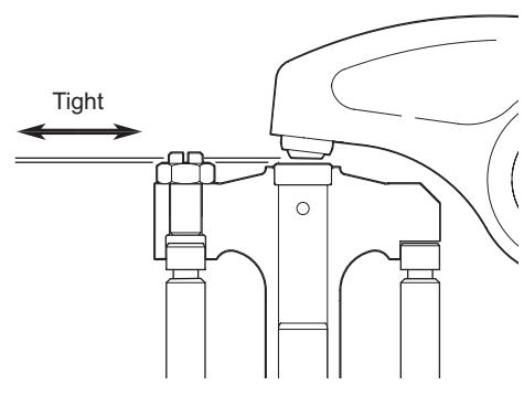
d) Loosen the rocker arm adjusting bolt and readjust the valve clearance by using the rocker arm adjusting bolt.
