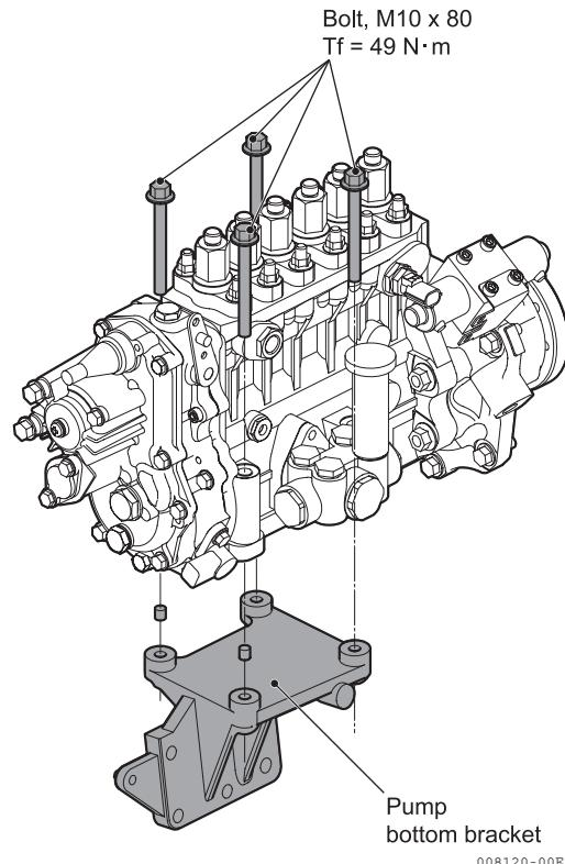
3) Tighten the pump bracket A with nuts while positioning by spring pins.
