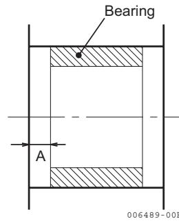
b) After press-fitting, check each bearing for distortion by measuring inner diameter of bearing.
