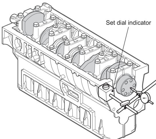
(Measurement of side clearance) 006614-00E
