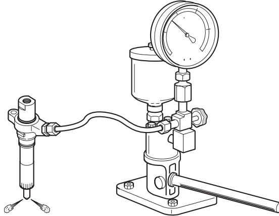
(Testing the valve opening pressure)
