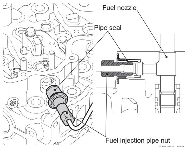
5) Finally tighten the retainer bolt for fuel injection nozzle to the specified torque.
