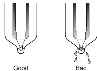
(Checking leakage from fuel injection nozzle)
