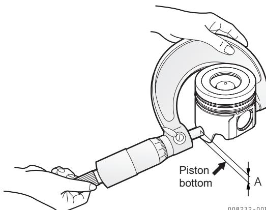
Selective pairing of cylinder liner and piston
