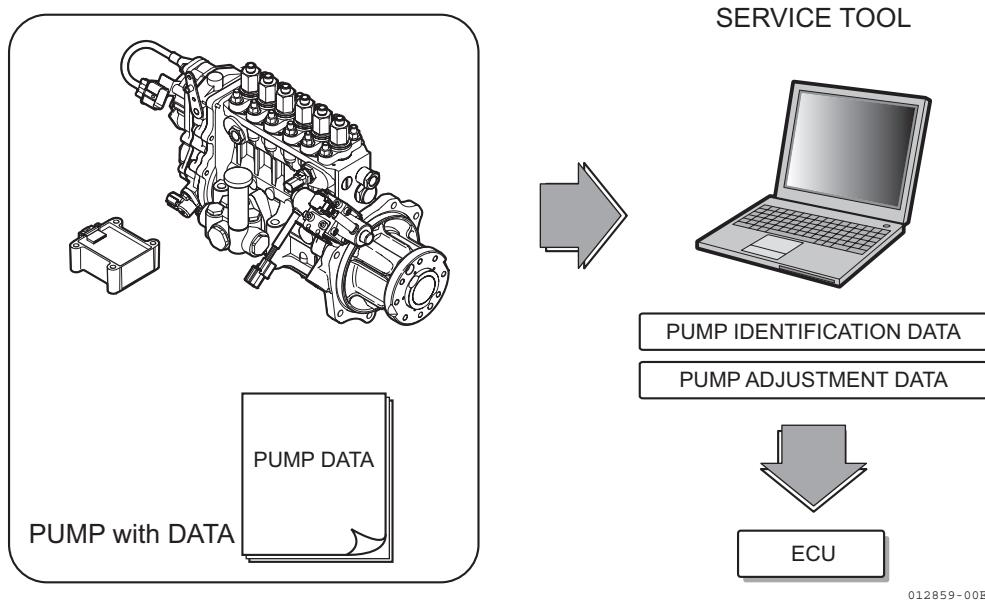
Figure below shows the ECU control data flow when **ECU replacement** is required. When an ECU is ordered to the factory, the ECU control data is selected according to the engine identification information such as engine serial number, pump serial number, etc. Then an ECU is provided directly by the factory. The data is stored into the production system network.
