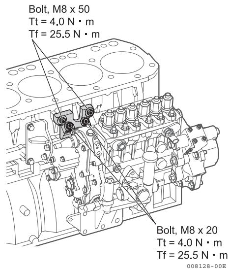
Finally tighten the bolts to the specified torque in the same order.
