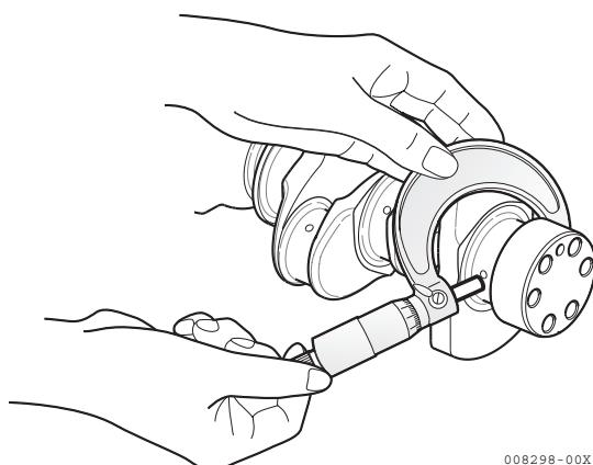
**(4) Checking the side clearance of a crankshaft**
