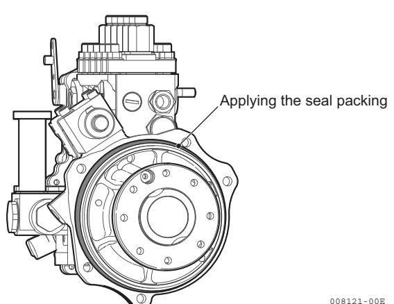
5) Install fuel pump assembly in the gear case and temporarily tighten the bolts (M8 - 3 pcs.) for timer housing and the dummy bolts (M8 - 2 pcs.).
