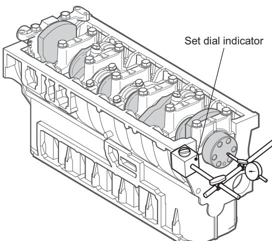
(Measurement of side clearance) 006614-00E
