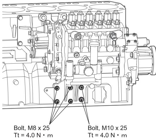
7) Tighten timer housing (fuel pump assembly) bolts to gear case. (without lube oil)
