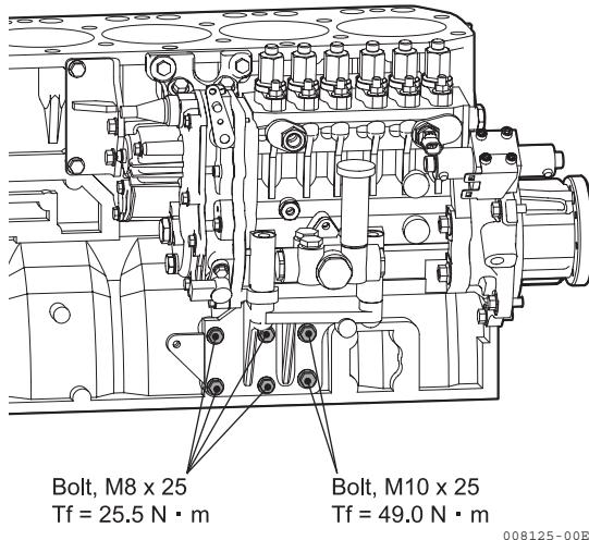
9) Remove the dummy bolts.
