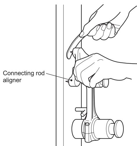
(Twist measurement using
