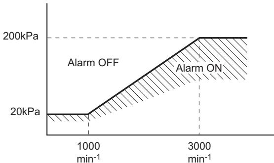
Alarm diagram of lube oil pressure
