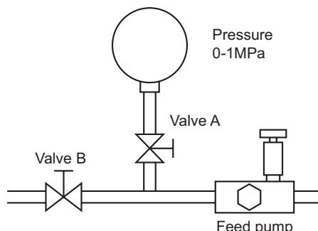
(Equipment for feed pump test)
