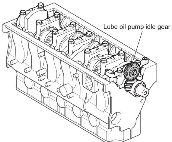
(Fitting of lube oil pump idle gear) 006615-00E
