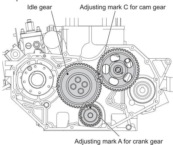
Adjusting mark A for crank gear
