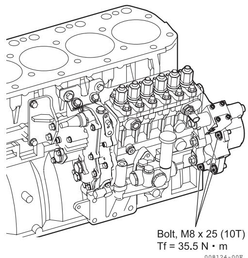
8) Tighten the bolts for pump bottom bracket.
