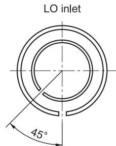
Position the ring closest to the compressor side as shown.
