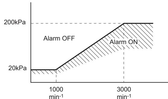
Alarm diagram of lube oil pressure
