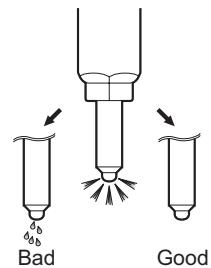
(Fuel drop check after injection test)
