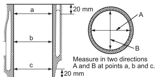
(Cylinder bore measurement positions)
