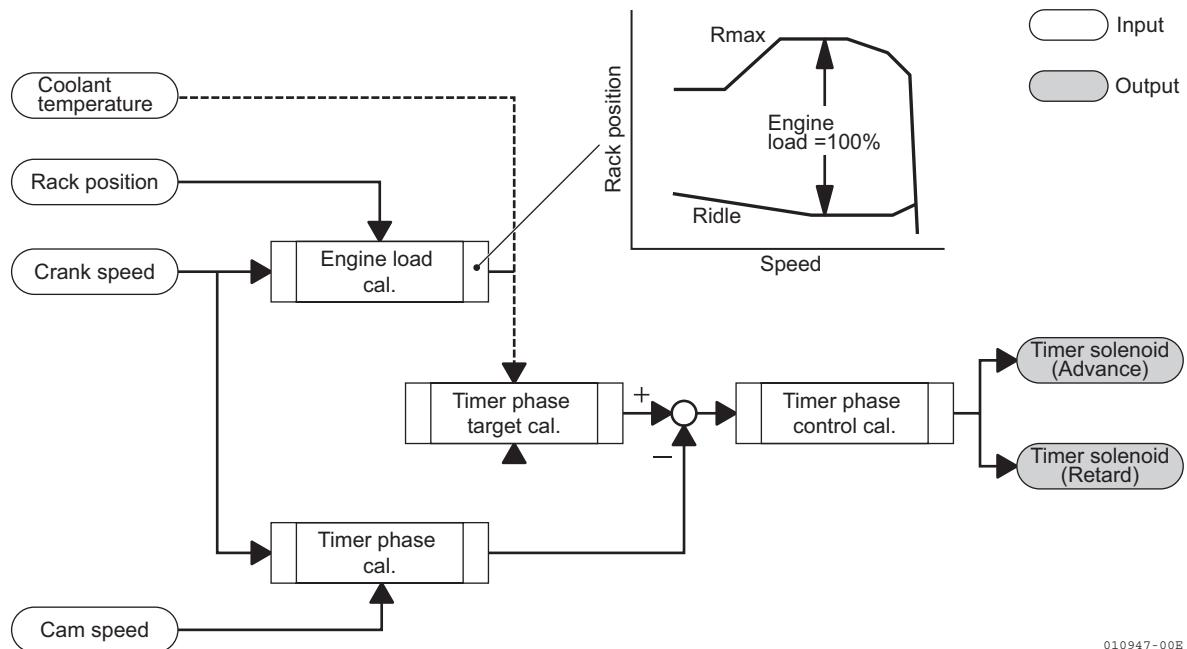
The timer phase is detected by two pulsar gears and is calculated by ECU from the deviation of two pulses.
