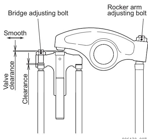
Standard valve clearance (mm)
