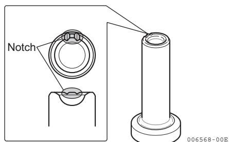
(2) Measure the outer diameter of the tappet, and replace if worn beyond the limit.
