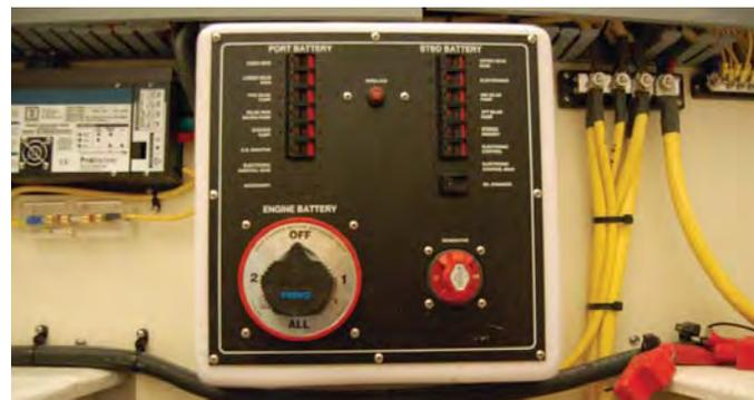
Figure 7.2 Battery Switch Panel
