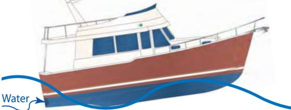
Then as the boat pitches down in the bow, some of the water drains into the muffler. Then on into the exhaust riser, and finally into the cylinders.
