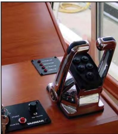
Fig. 11.3 You will find an engine control at the helm station. The control contains the function of synchronization, throttle, shift, and monitoring of the engine controls. Moving the lever forward engages the forward gear and increases the throttle, as moving backwards does reverse.
