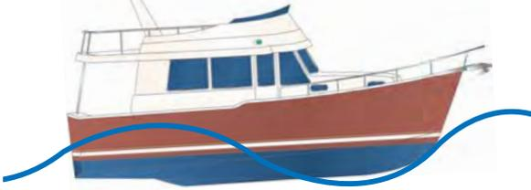
The high water level plus the surging action caused by the rocking motion, can result in water entering the exhaust and flowing to the header.
