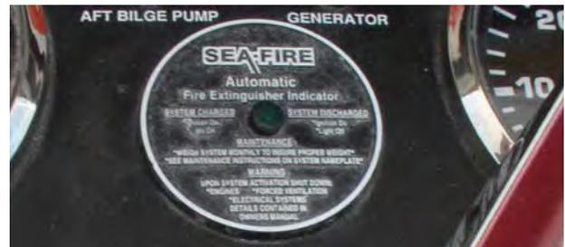
Figure 7.11 Fire Alarm Monitor
